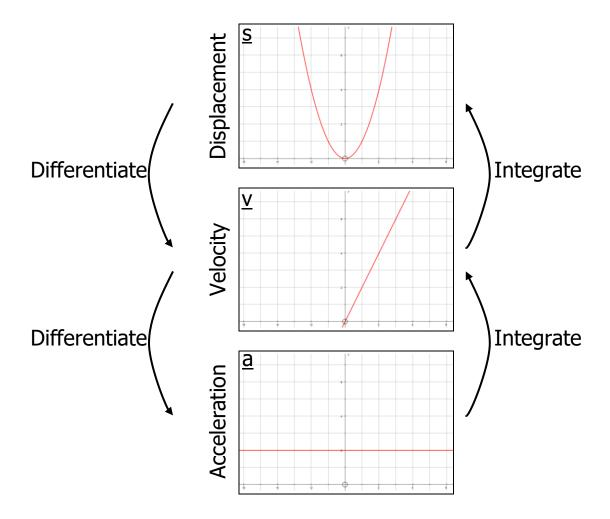
On the velocity-time graph below, the gradient  $(\frac{\partial v}{\partial x})$  of the sloped section is acceleration and the area under the graph  $(\int v \, \partial x)$  is the distance travelled.
